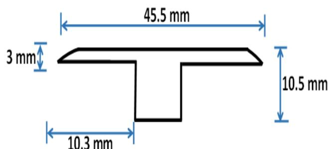
**Note:-** Laminate Flooring can be installed in a single room / area up to 36 linear feet in length or width. Installations in rooms / areas over 36 linear feet in length or width must use T-moldings. Otherwise, the warranty will be void.
