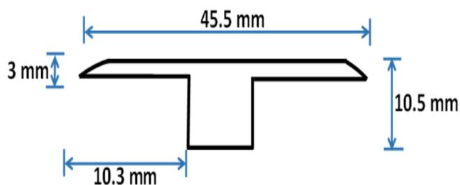
**Note:-** Laminate Flooring can be installed in a single room / area up to 36 linear feet in length or width. Installations in rooms / areas over 36 linear feet in length or width must use T-moldings. Otherwise, the warranty will be void.
