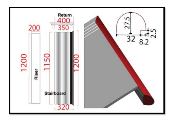
This picture depicts a side view of a stair tread and riser. The Luxury Vinyl Tread (LVT) nose piece is installed and glued into place, and joined with a piece of standard stair planking that has been cut to cover the remainder of the tread. A riser cover can then be affixed to finish the step.
